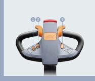
FREI multi-function tiller 1: Forks move forward / backward 2: Forks lifting / lowering 3: Forks tilt forward / backward
