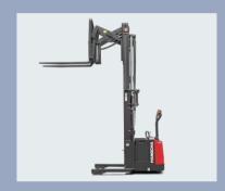
Travel speed is lowered automatically when fork is lifted to specified height
