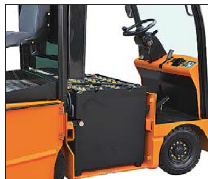
Side-exchange battery design is convenient for changing battery.
