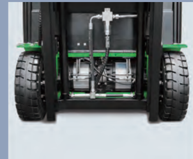
Dual Front AC Driving Motors
